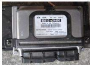
Engine control unit
